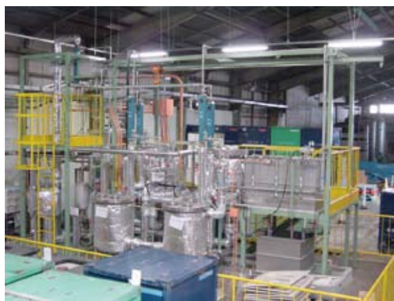
FRP recycling demonstration plant
