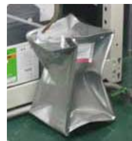
Equipment broken due to depressurization
